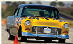
Lowers your Ti-Five 3-4". Caster has been increased to provide improved stability at speed & greater tire contact
